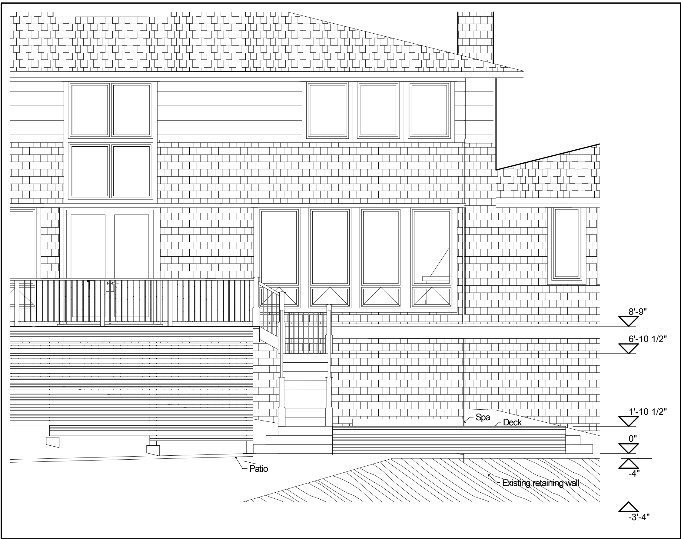
#2 Stairs, Spa, and Deck East Elevation 1/4" = 1'
