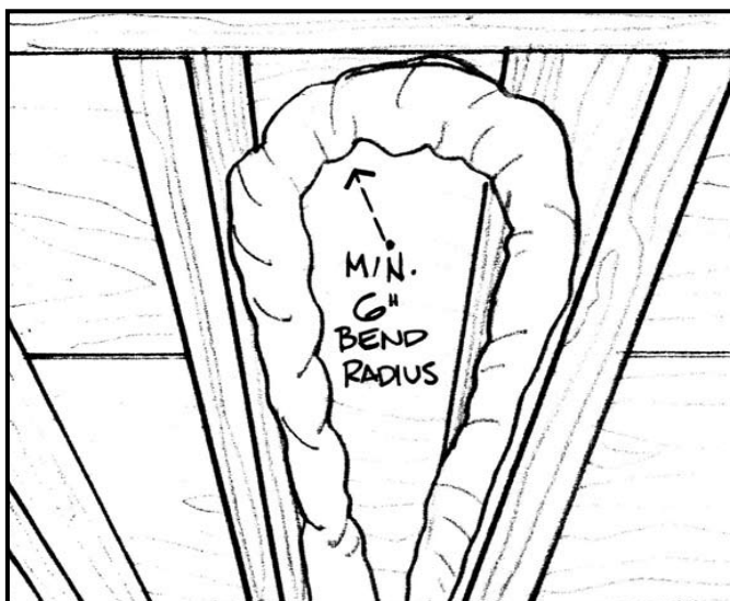
Fig. 46 - 6" minimum radius on bends
